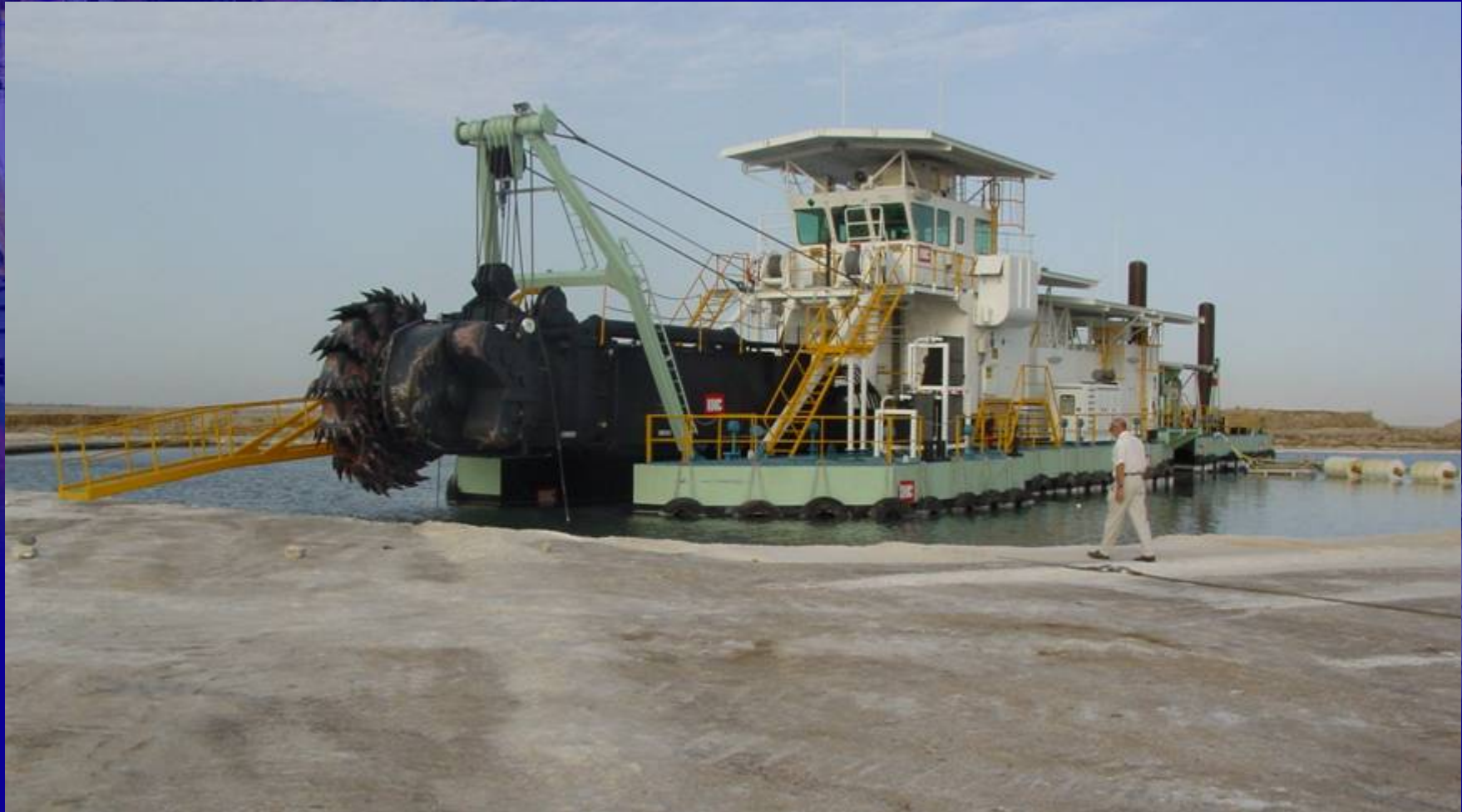
Wheel suction dredger mining in rock salt (Saudi Arabia)
