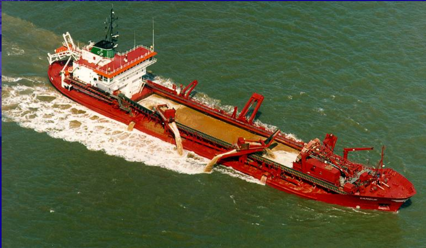
Gravel hopper dredger mining sand & gravel offshore (North Sea)
